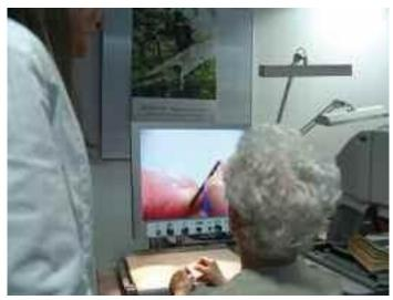
Figure 15.11. Threading a needle using a video magnifier.
